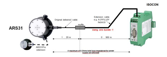
For example, extension of 100 m with a 0.5 mm<sup>2</sup> cable of 73.2  $\Omega$ /km loop resistance and parallel connection of 4 cores each:
