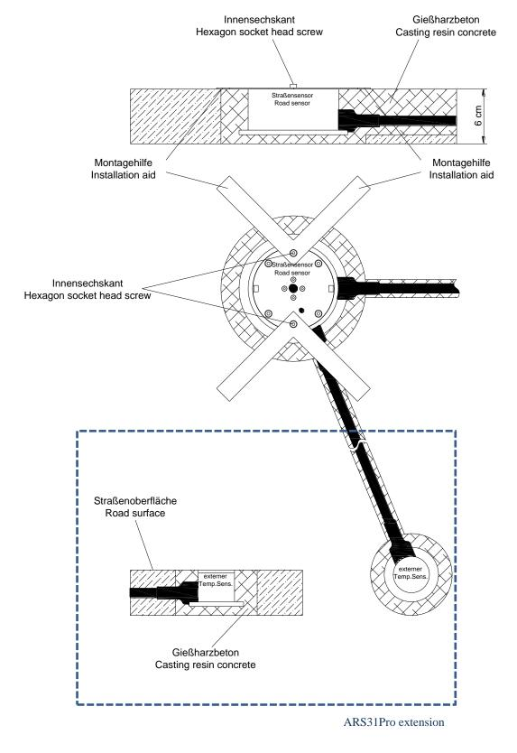
Illustration 3: Installing the ARS31PRO-UMB/ARS31-UMB
