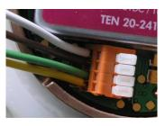
The data and power supply cables are connected via a 4-pole terminal block. Cable type LI-2YCYv2X2X0.5 is used.
