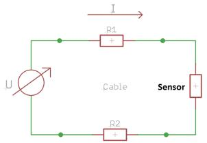
R1 + R2 = loop resistance U = Voltage in the cabinet at the end of the cable (24V) U<sub>S</sub> = voltage at the sensor I = supply current I is calculated with the equation  $I^2 - I \frac{U}{(R1+R2)} + \frac{P}{(R1+R2)} = 0$  $\frac{U}{(R1+R2)} - \sqrt{\left(\frac{U}{(R1+R2)}\right)^2 - 4*\frac{P}{(R1+R2)}}$
