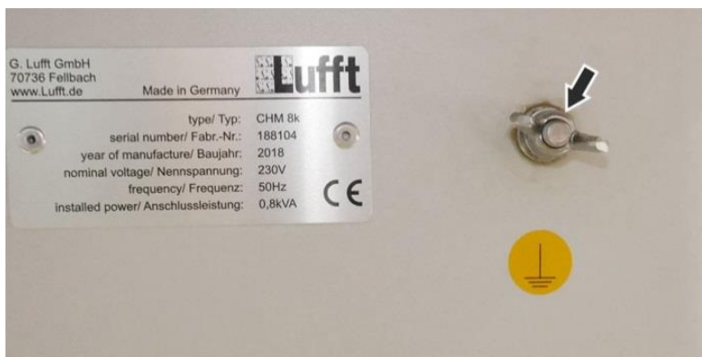
Figure 12 Grounding connection at pedestal of device.
