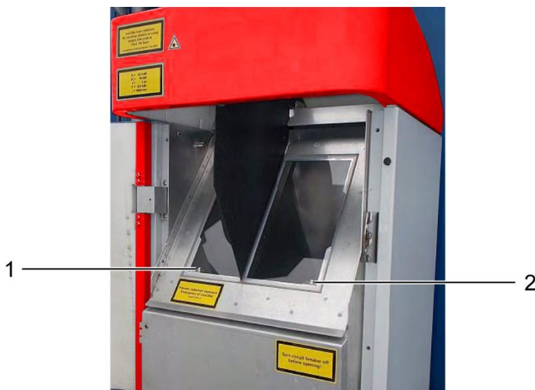
Figure 29 Windows to be cleaned.
