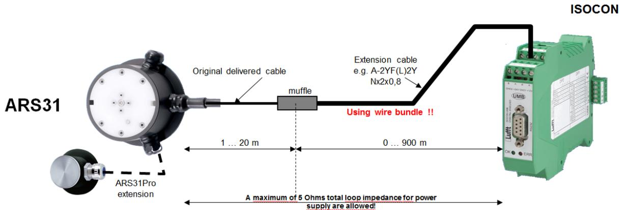
For example, extension of 100 m with a 0.5 mm<sup>2</sup> cable of 73.2 Ω/km loop resistance and parallel connection of 4 cores each:
