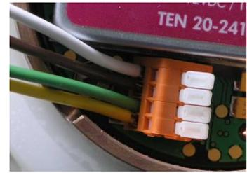
The data and power supply cables are connected via a 4-pole terminal block. Cable type LI-2YCYv2X2X0.5 is used.
