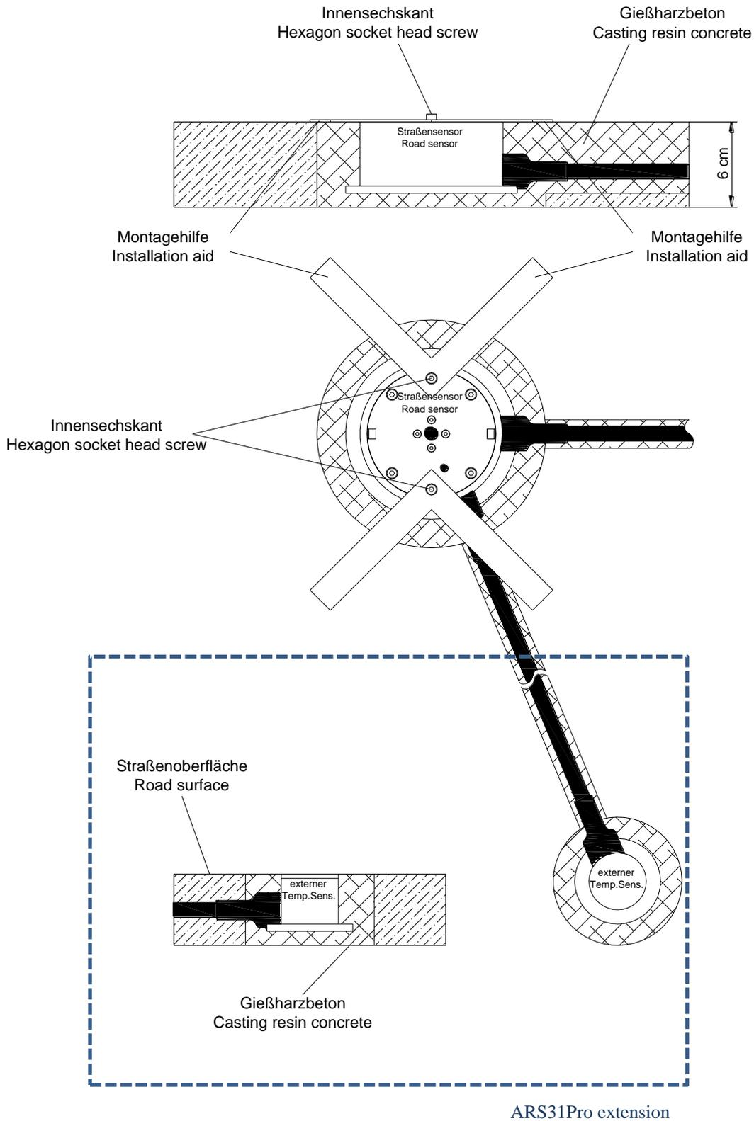
**Illustration 3: Installing the ARS31PRO-UMB/ARS31-UMB**
