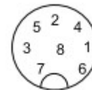
III 26: View on solder connection of the cable socket
